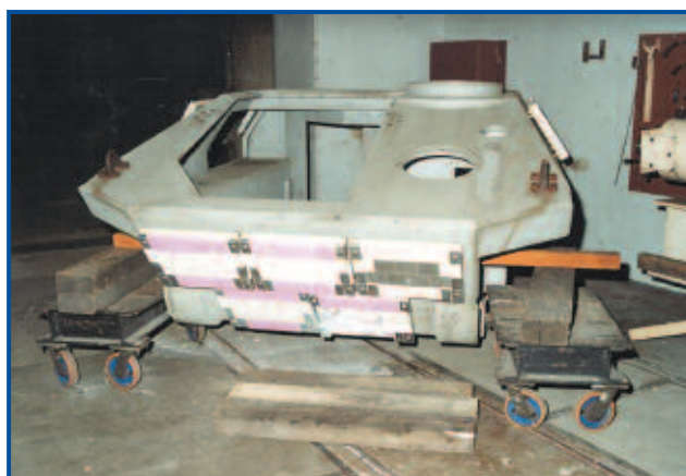
Vehicle hull with add-on armour prior to ballistic testing.
