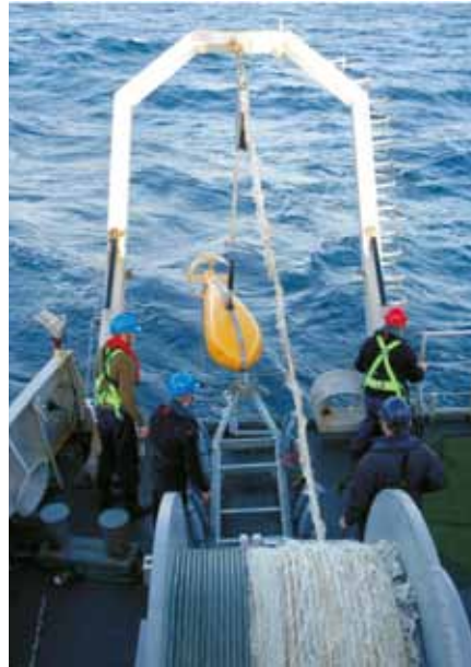
Socrates2 suspended from the A frame of the HNLMS Mercur during calibration sea trials
