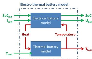
Figure 1 Electro-thermal battery modelling structure
