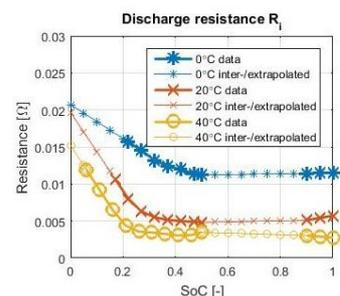
Figure 2 Example of a SoC- and Temperature-dependent battery model parameter
