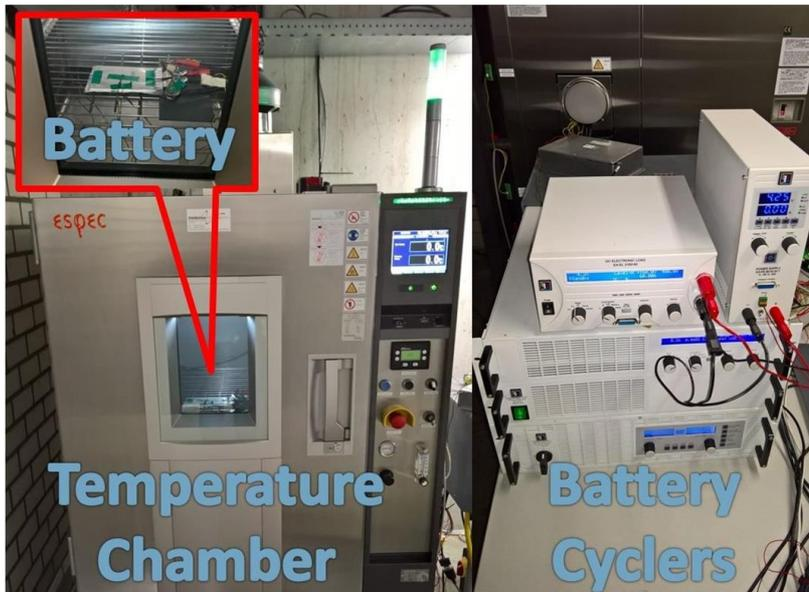
Figure 3 Battery testing facility for cells and modules, coupled to a temperature chamber
