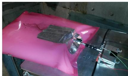
Figure 5 Example of an abuse test with gas analysis
