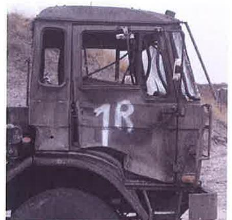
Structural deformation in old truck cabin after a road side IED blast test.
